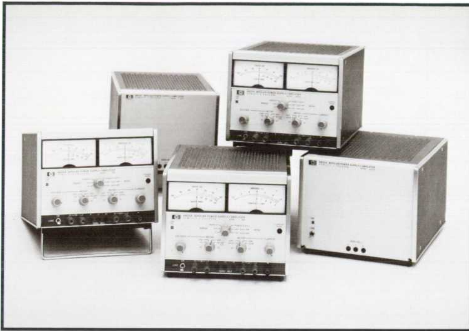
Fig. 1. New Bipolar Power Supply/Amplifiers are made in two versions: one with front-panel meters and controls for bench use and one with blank front panels for systems use. All have 0.01% line and load regulation but respond quickly (<0.1 ms) to external voltage or resistance programming commands.
