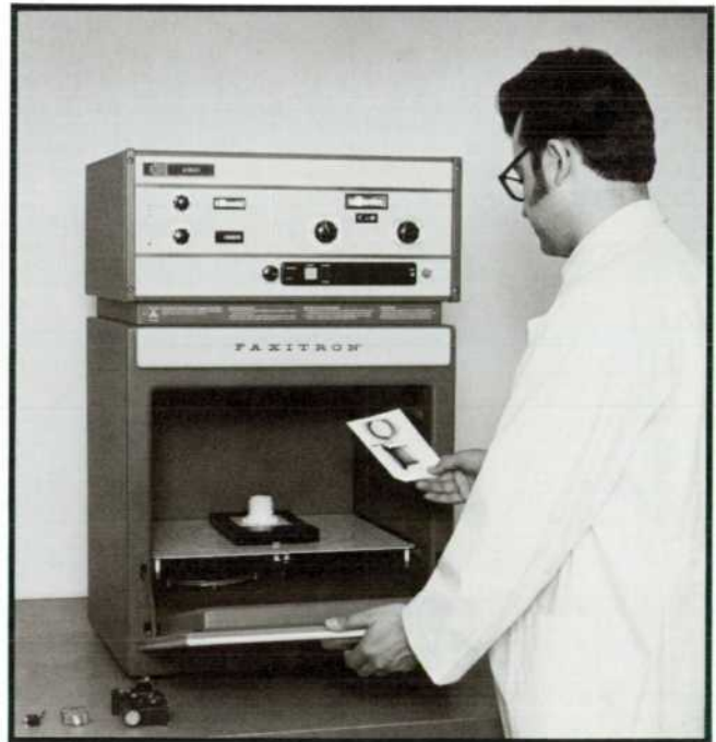
Fig. 1. X-ray system developed by the Field Emission Corporation, now Hewlett-Packard's McMinnville Division, has a lead-shielded enclosure with electrical door interlocks to ensure safety for everyday lab applications. It uses a simple, self-rectified circuit for the x-ray tube. The basic unit, with a film-to-source distance of 24 inches, covers film sizes up to 8 × 10 inches. Film to source distances up to 66 inches can be obtained with cabinet extensions.
